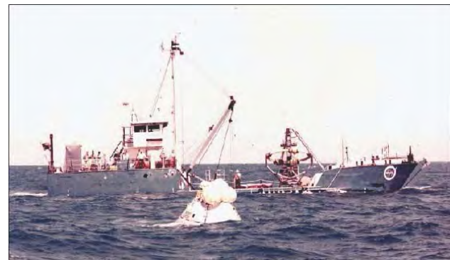
NASA Motor Vessel (MV) Retriever was a Landing Craft Utility (LCU) built for the U.S. Army in 1953. After modifications it arrived at its Seabrook, Texas docking facility near the NASA Manned Spacecraft Center (MSC) in June 1963.
