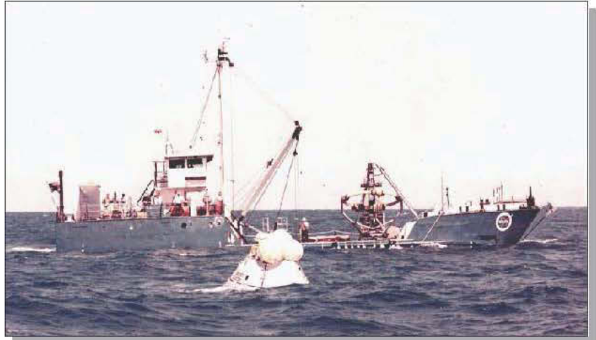
The NASA Motor Vessel (MV) Retriever was a Landing Craft Utility (LCU) built for the U.S. Army in 1953. LCU-15301 was acquired from the Army in 1963. After modifications (the sides of the vessel's midsection were cut down, a new bridge built, and a hoist added), it arrived at its Seabrook, Texas docking facility near the NASA Manned Spacecraft Center (MSC) in June 1963. The modified Army LCU, painted NASA blue and white, was named "Retriever" to signify its mission of recovering spacecraft. The LCU was selected because its shallow draft, which allowed it to operate in Galveston Bay as well as in the Gulf of Mexico off of Galveston, Texas.
