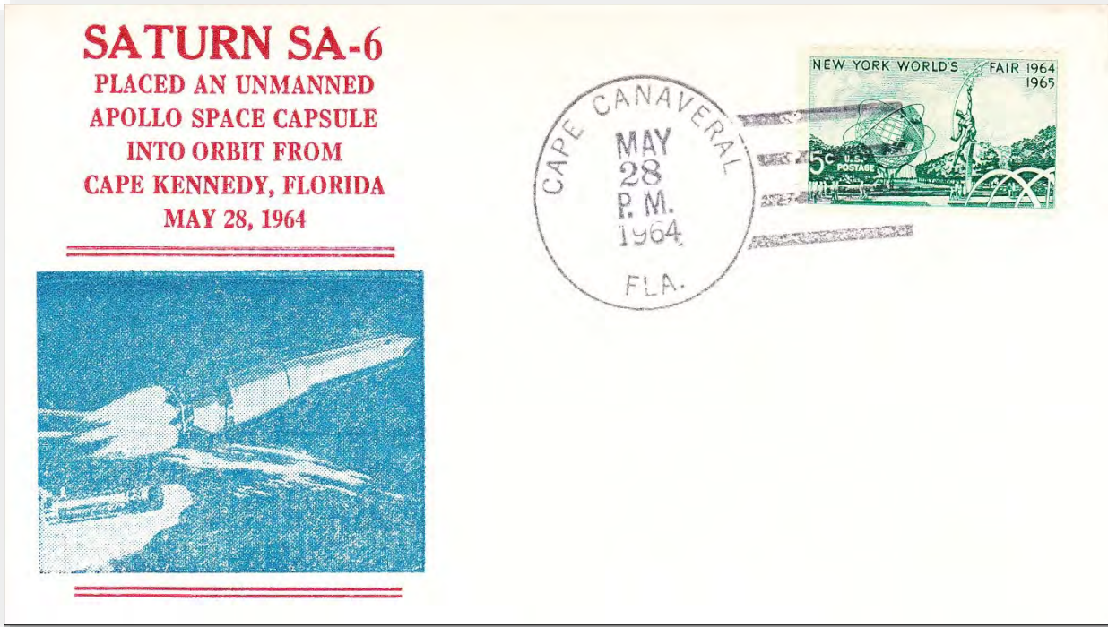
First to fly an Apollo boilerplate capsule. The first stage burned 2.7 seconds longer to compensate for engine number 8 which shut off early. Postflight cause was quickly located with no further delay.
